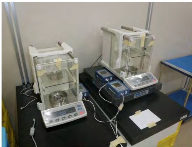
Fig.1 Alignment of balance and weighing environment logger
